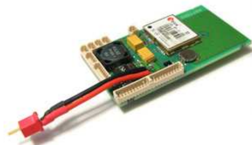
Figure 2. Paparazzi Tiny Board
